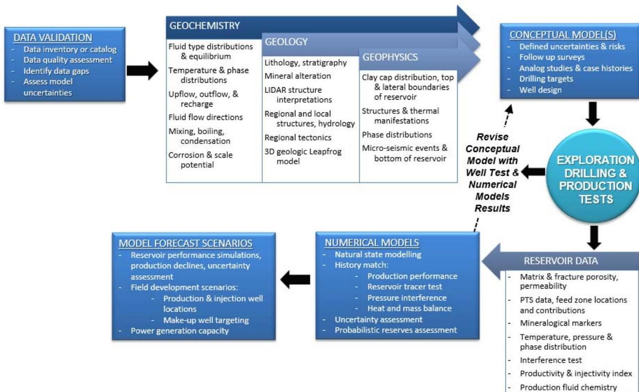
Figure 1. Illustration of resource evaluation process
