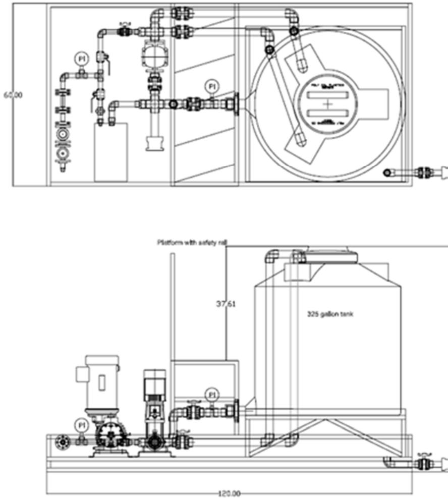
Figure 2 Thermochem Rapid-Injection Pulse Skid (RIPS)
