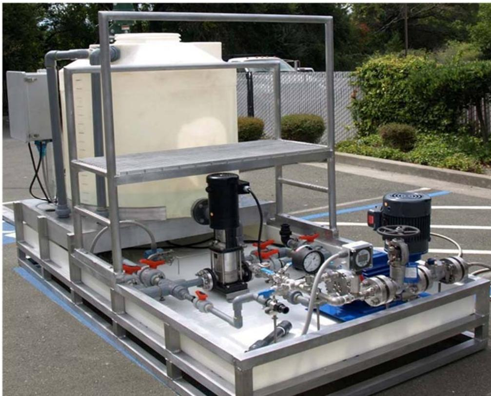
**Figure 1**      **Thermochem Rapid-Pulse Tracer Injection Skid (RIPS)**
